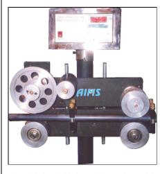
The coder is installed in front of the extrusion machine where the extruded pipe passes over the support rollers & below the print head where it gets printed on-line during production after every preset length repeatedly.
