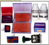
For the basic system, the grooved rubber stereos are push fitted into the grooved base mat to form the message of 3 to 5 lines. Then it can be inked manually on the inkpad & stamped onto the substrate to get a permanent printing.
