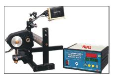
The coder is installed on the FFS machine & the film goes over the roller where it gets coded at the desired location on-line during production.
